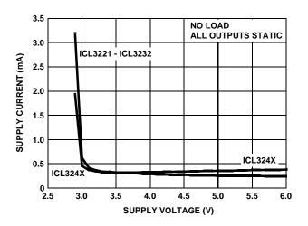
FIGURE 18. SUPPLY CURRENT vs SUPPLY VOLTAGE
