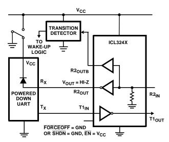
FIGURE 3. DISABLED RECEIVERS PREVENT POWER DRAIN
