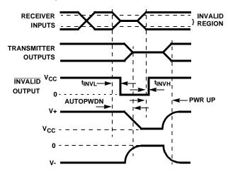
FIGURE 7. AUTOMATIC POWERDOWN AND INVALID TIMING DIAGRAMS
