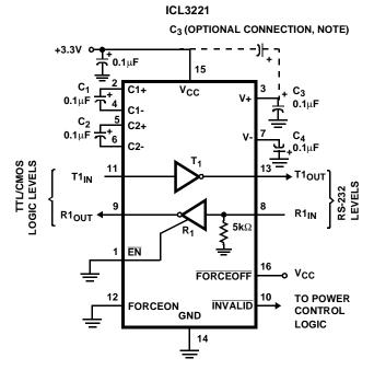
NOTE: THE NEGATIVE TERMINAL OF  $\mathrm{C_3}$  CAN BE CONNECTED TO EITHER  $\mathrm{V_{CC}}$  OR GND
