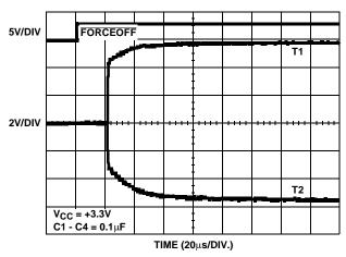
FIGURE 8. TRANSMITTER OUTPUTS WHEN EXITING POWERDOWN
