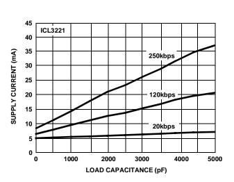
FIGURE 15. SUPPLY CURRENT VS LOAD CAPACITANCE WHEN TRANSMITTING DATA
