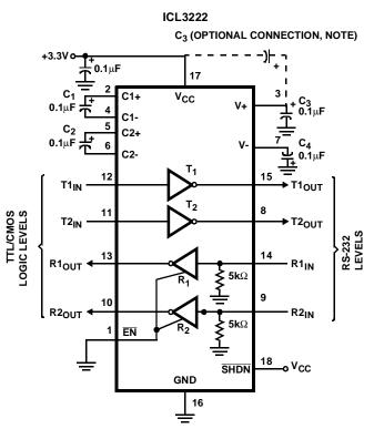
NOTE: THE NEGATIVE TERMINAL OF  $\ensuremath{\text{C}_3}$  Can be connected to either  $\ensuremath{\text{V}_{\text{CC}}}$  or gnd
